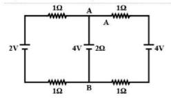
The potential difference between the points A and B for the electric circuit shown in figure. is:
