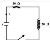
The switch is closed at t=0. The time after which the rate of dissipation of energy in the resistor is equal to rate at which energy is being stored in the inductor is :
